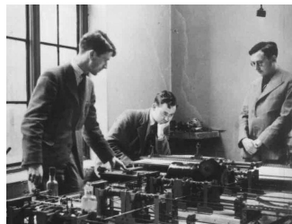
The old way... Wilkes (right) and colleagues in the 1930s with a mechanical analogue computer that was designed to solve differential equations. Analogue computers can also be electrical and may still be used for some purposes
